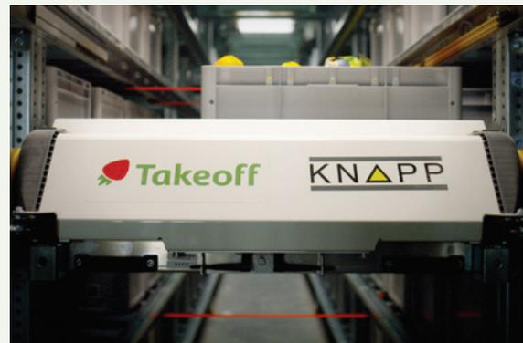
Systems developed by Takeoff Technologies use small shuttles such as the one pictured to move frequently purchased goods through Micro Fulfillment Centers, thereby making it more convenient and cost effective for grocers to engage in e-commerce. *Courtesy Takeoff Technologies.* ■
