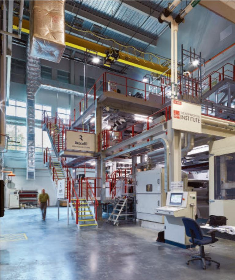
This nonwoven spunbond extruder machine occupies the first floor of the Center for Technology & Innovation. It's used by N.C. State's Nonwovens Institute (NWI), a partnership between industry, government and academia that's affiliated with the N.C. State College of Textiles. The machine, which is roughly 52 feet tall and 170 feet long, produces prototypes of fabrics that are used in a variety of consumer, medical and industrial applications.
